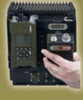
handheld radio, there is a slot on the amplifier block for the way for the user to adapt (extend) the properties of the vehicular radio to specific deployment. The electromechanical concept that can integrate electronics of different types. There is, for example, MM40W, which implements a MANET-type broadband radio. By installing this module, the properties of the radio are extended by a second independent radio channel (L-band or S-band (adjustable from 5 to 40 MHz)
