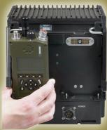
The RF40V vehicular radio consists of the RF40 handheld radio and an amplifier block into which the radio is docked. Docking of the radio provides its firm mechanical attachment and system interconnection through a multi-pin nut connector and power connector on the back of the radio.
