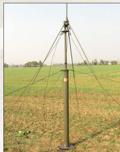
Obr. 2: Instalace antény VHF3076P na stožár MT1790
