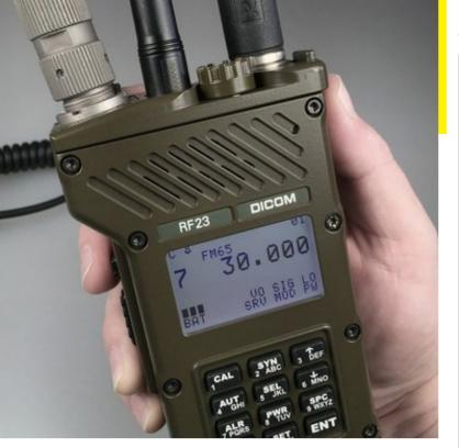
RF23 handheld multiband transceiver with increased resistance against radio-electronic warfare intended for squad/team, platoon and company operation is part of the RF20 tactical radios family.
